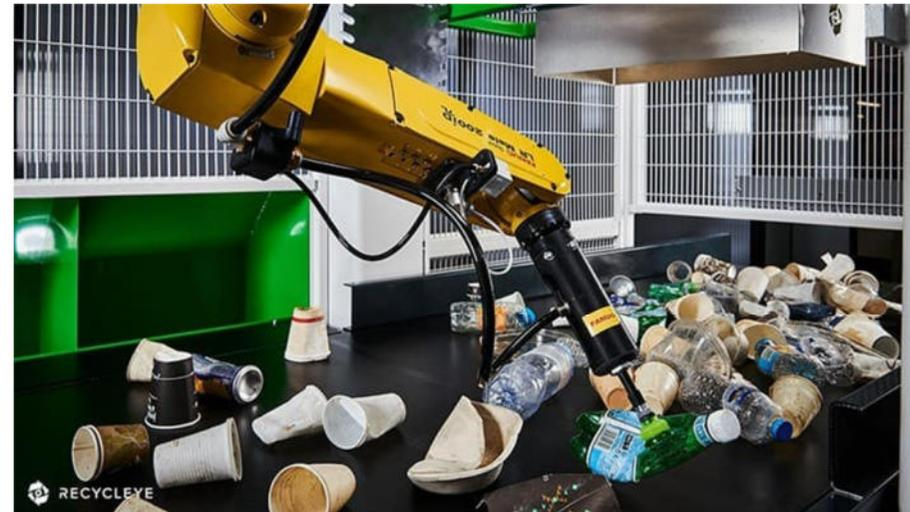
AMP Cortex™ - A robotics system that performs tasks of sorting, picking and placing material
